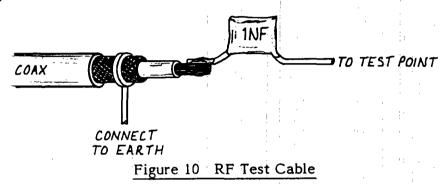
Note: Before using the test cable, ensure the coax braid is connected to an earth point on the PCB.
