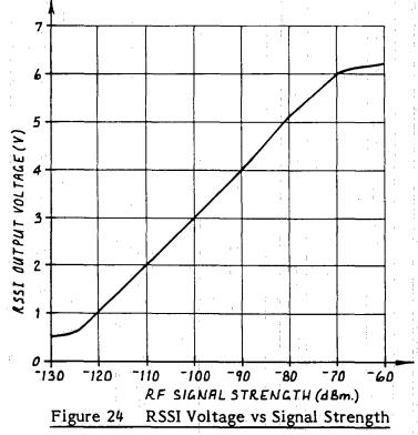
When fitted, the RSSI also gives the capability of high level signal strength muting, which may be selected on PL104 (refer to Section 4.4). The mute threshold may be set between -115dBm and -70dBm on RV104.
