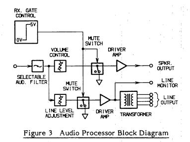
The recovered audio on pin 9 of IC301 is processed in a third order elliptic active filter to give the required response. Linking (PL101 & PL103) is available to give either a flat or de-emphasised audio response, with de-emphasis giving a 6dB/octave roll off. The output of IC101 is split to provide separate paths for the speaker and line outputs.
