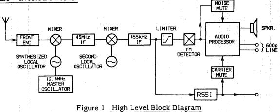
The T885 receiver consists of a number of distinct stages: the front end, mixer, synthesised local oscillator, IF, audio processor, mute (squelch), regulator circuits and received signal strength indicator (RSSI). These stages are clearly identifiable in Figure 1. Refer to the Circuit Diagrams at the rear of the Manual for further detail.
