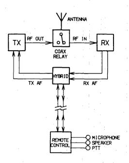
Figure 18 Remote Line Controlled Base Station
