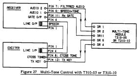
An alternative configuration is to send speech plus tone along the 600 ohm line and carry out the detection on the transmitter audio. However, this would require the 300Hz high pass filter formed by Q109 to be linked out, thus degrading the residual hum and noise performance by 10dB.
