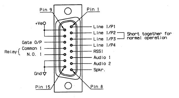
Figure 15 D-Range Wiring - Rear View
