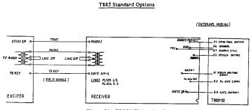
Figure 26 CTCSS Wiring Detail
