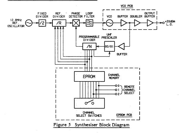
The synthesiser employs a phase-locked loop (PLL) to lock a VCO to a given reference frequency.
