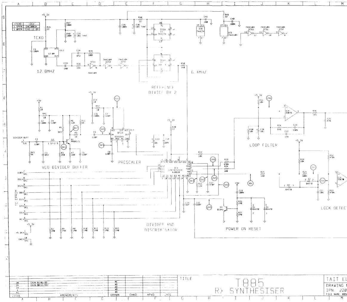
DIAGRAM 14 SYNTHESISER CIRCUIT DIAGRAM
