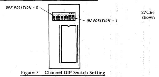
The PGM800 software used to programme the EPROM will present the user with a DIP switch code for each channel address. For example, channel 124 will be assigned a switch code of X0000011, in which case the switches should be set as shown in Figure 7, i.e. **0**0000011.
