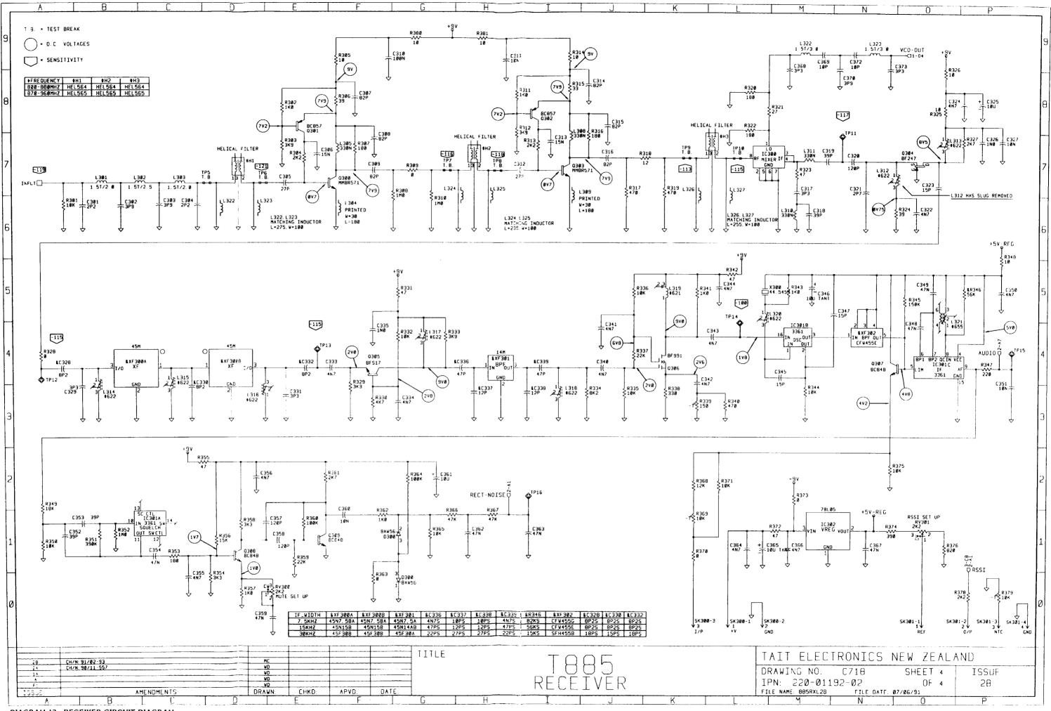
DIAGRAM 12 RECEIVER CIRCUIT DIAGRAM
